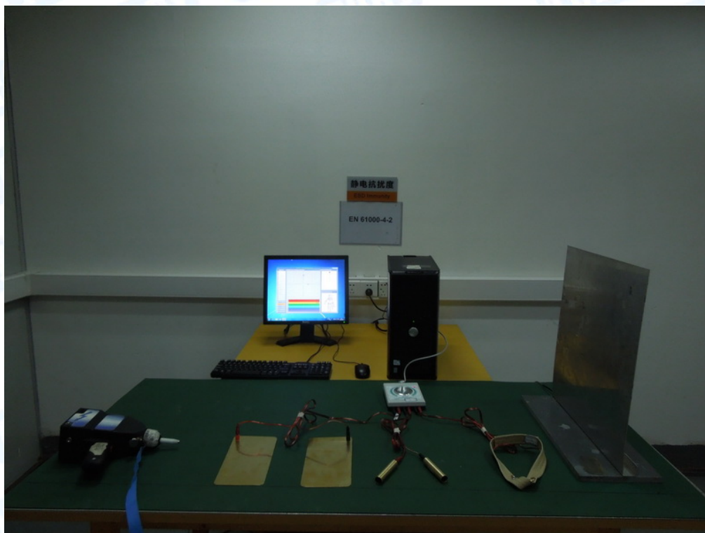
Photo 3 Electrostatic Discharge Test Setup
